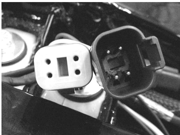
Figure 5—Disconnect and Remove Coil Harness
