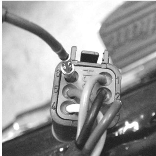
Figure 4—Blue Wire Installation
