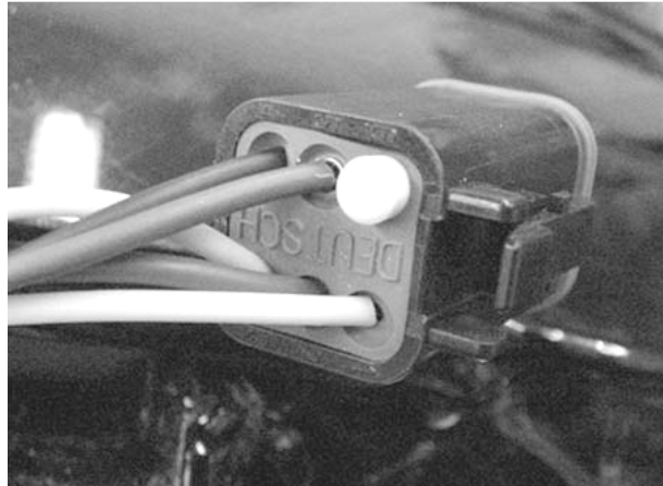
Figure 7—Finished Coil Harness Connector
