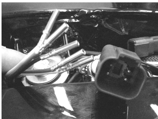
Figure 6—Thread New Coil Harness Near Factory Connector
