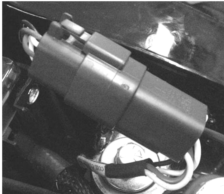
Figure 10—Finished Main Harness Connection
