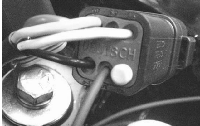
Figure 9—Finished Main Harness Connector
