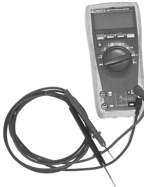
Figure 4—Multi-Meter; useful for circuit diagnosis
